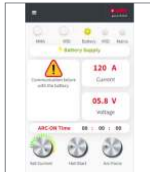
COMMUNICATION FAILURE BETWEEN BATTERY AND POWER SOURCE
