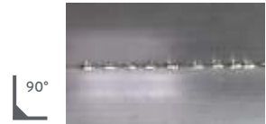
Corner spot welding thickness 0,6 mm
