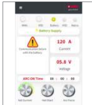
COMMUNICATION FAILURE BETWEEN BATTERY AND POWER SOURCE
